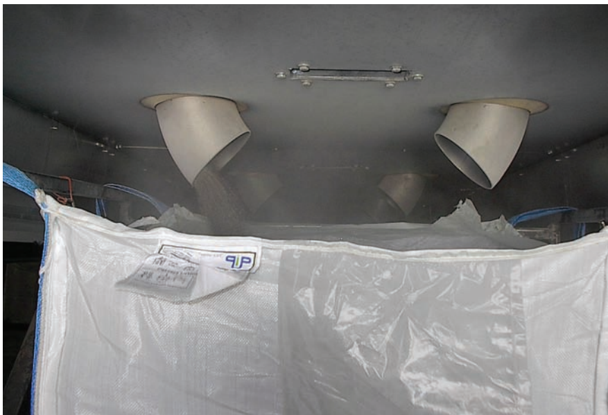
Two dust pick-ups capture fugitive dust created as an ingredient discharges from a hopper through a short length of tube into the batch bag.
